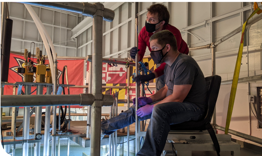
Mike Hottinger and Luke Gilde assemble used fuel into a bundle in the MUTR pool.
